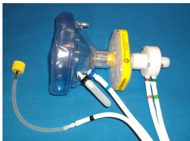
As before but with filter added Note blanking plug on black mask port.
