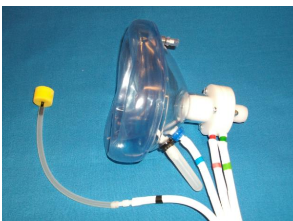
Adult mask (1 use) set for Anterior test. Note blanking plug on black mask port.
